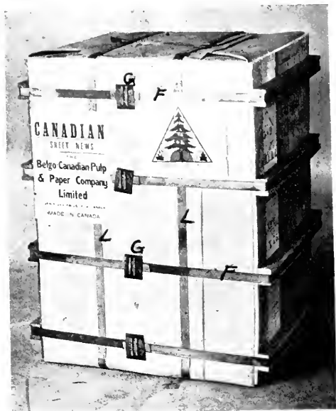
3.—Side view of bale showing buckle pin arrangement, extra iron bands and wrapper strip—(strips of wrapper protecting edge of paper where iron cross bands press on edges are under the wrapper strip.)
